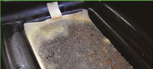
The Filter is the KEY to the system – it not only traps particles down to 50 micron, it also contains millions of Rozone microbes.
