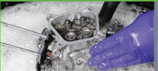
Heated to 42°C, the microbes become active in the ROWash solution and eat the oil and grease turning them into CO<sup>2</sup> and water – effectively recycling the fluid.
